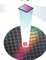
Wafer on which CFA is formed
