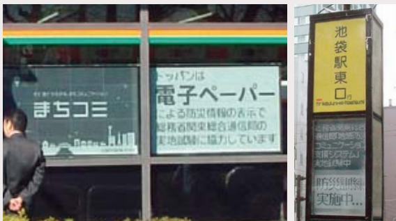
Left: Large-size electronic-paper signage at Toshima Post Office Right: Electronic-paper signage mounted on a bus stop sign at Higashi Ikebukuro 2-chome
